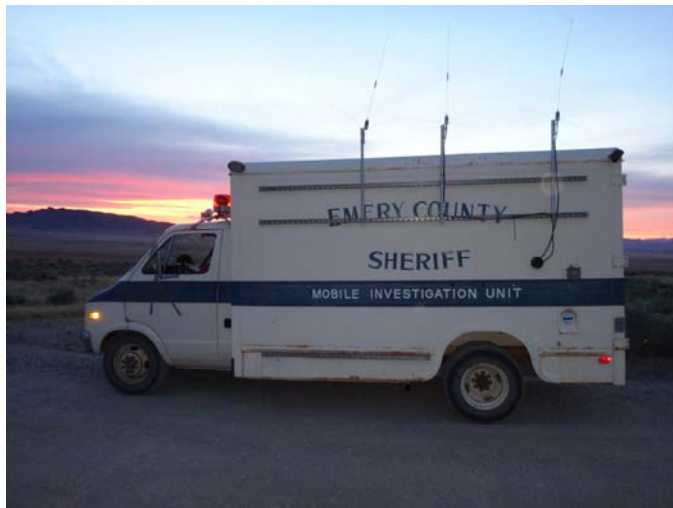
Fig. 11 "The Rover" carries VHF mobile communication equipment, six crossed dipole antennas, and two operators. Here it is just about ready to start the night.
