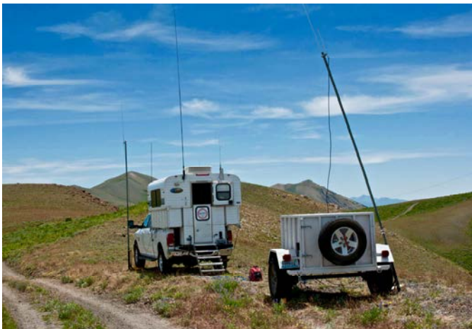
Fig. 6. Nevada ham operators provide communication access in some of the remotest areas of the Pony Express Re-Ride. This photo shows the 2018 setup at the peak of the Austin Summit. The 2 tall poles have dual band J poles antennas; one set to communicate on the VHF simplex frequency (146.55MHz) and one set to communicate with the Fallon repeater (147.345MHz). There are two dipoles off to the right of the photo and the 19 foot whip on the camper shell was used for various HF frequencies through an autotuner.
