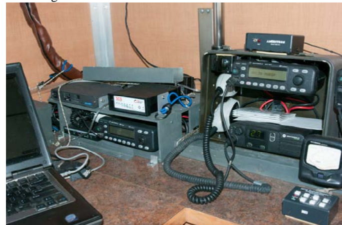
Fig. 8. Three of the modems are shown. These include the SCS Pactor 3/4 modem, the RapidM RM2 modem for the military M110A mode, and the Kantronics Packet Modem. A modem for Winmor is behind the computer.
